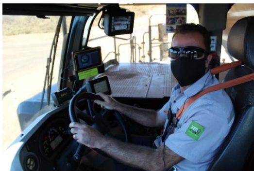
Image 3: Fatigue detection system in operation
